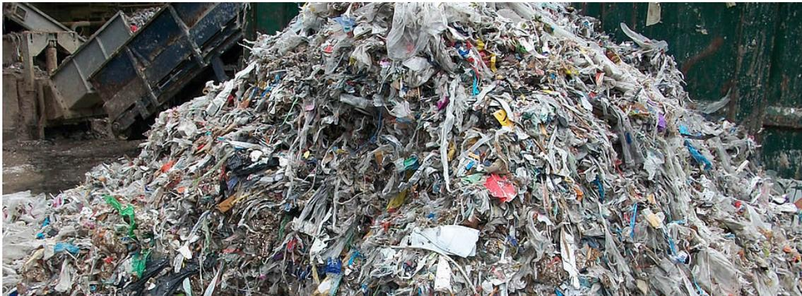
The [LIFE ECO-PULPLAST](#) project aims at demonstrating the possibility to recycle pulper waste – the industrial waste of paper mills that use recovered paper – in the manufacturing of eco-sustainable plastic pallets.
