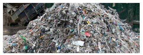
The <u>LIFE ECO-PULPLAST</u> project aims at demonstrating the possibility to recycle pulper waste – the industrial waste of paper mills that use recovered paper – in the manufacturing of eco-sustainable plastic pallets.
